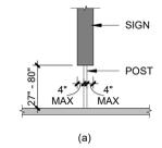
FIGURE 307.3 POST MOUNTED PROTRUDING OBJECTS
