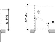
FIGURE 404.2.3.3 FRONT APPROACH, PUSH SIDE, W/ CLOSER AND LATCH
