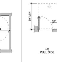
FIGURE 404.2.3.5 MANEUVERING CLEARANCES AT RECESSED DOOR AND GATES
